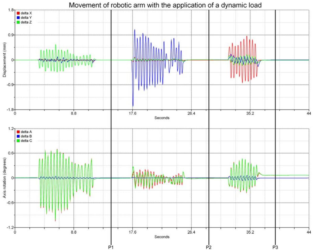
**Figure 82 - Top: Position oscillation with dynamic load applied. Down: Angle oscillation with dynamic load applied. Horizontal axis displays time in seconds. On the top graphic the vertical axis displays the robot arm displacement in millimetres, the bottom graphic the robot arm displacement in degrees.**
