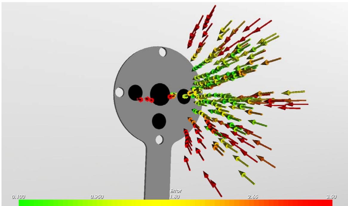
**Figure 74 - Spatial representation of the depth error growth with the camera distance and orientation.**
