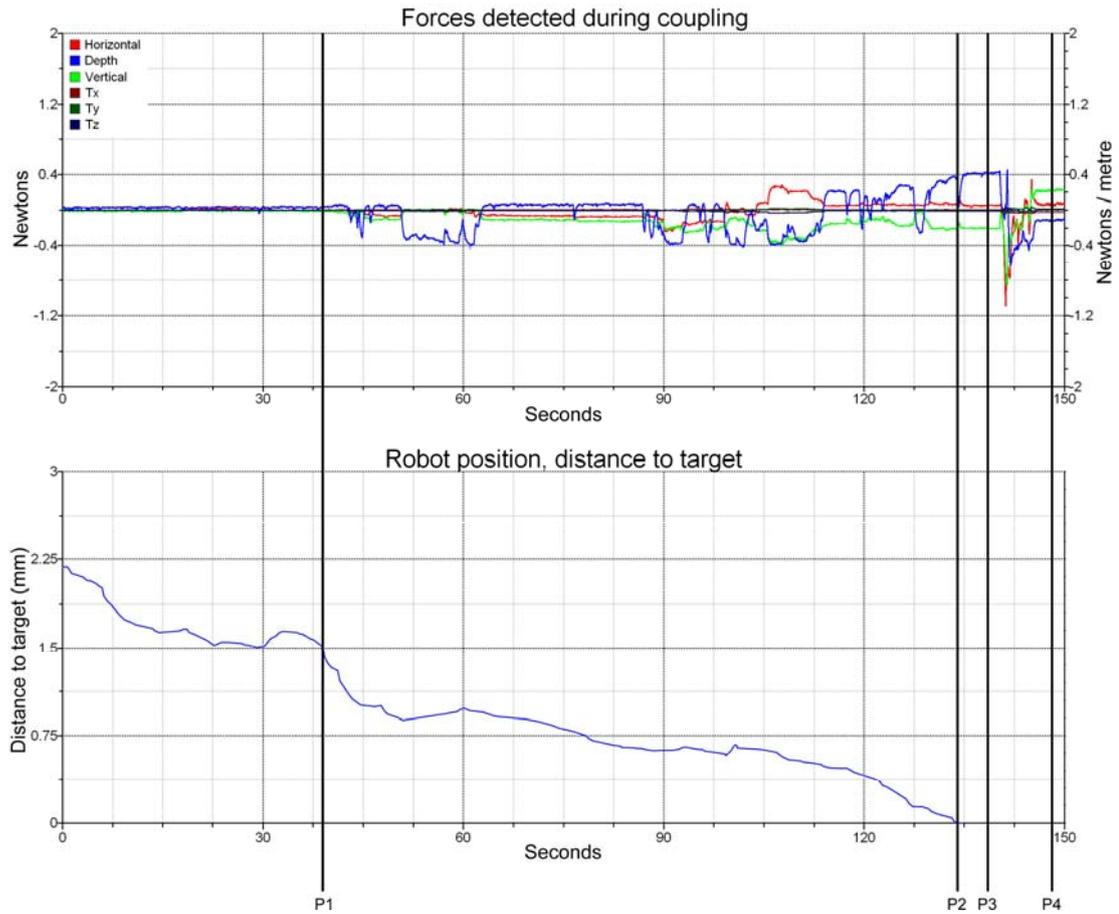
**Figure 79 – Top: Detected forces by the FTS. Bottom: Distance from the target as indicated by the robot controller. Horizontal axis displays time in seconds. On the top graphic the vertical axis contains the measured force in Newton as well as the torques in Newton / metre, the bottom graphic the distance to the target in millimetres.**
