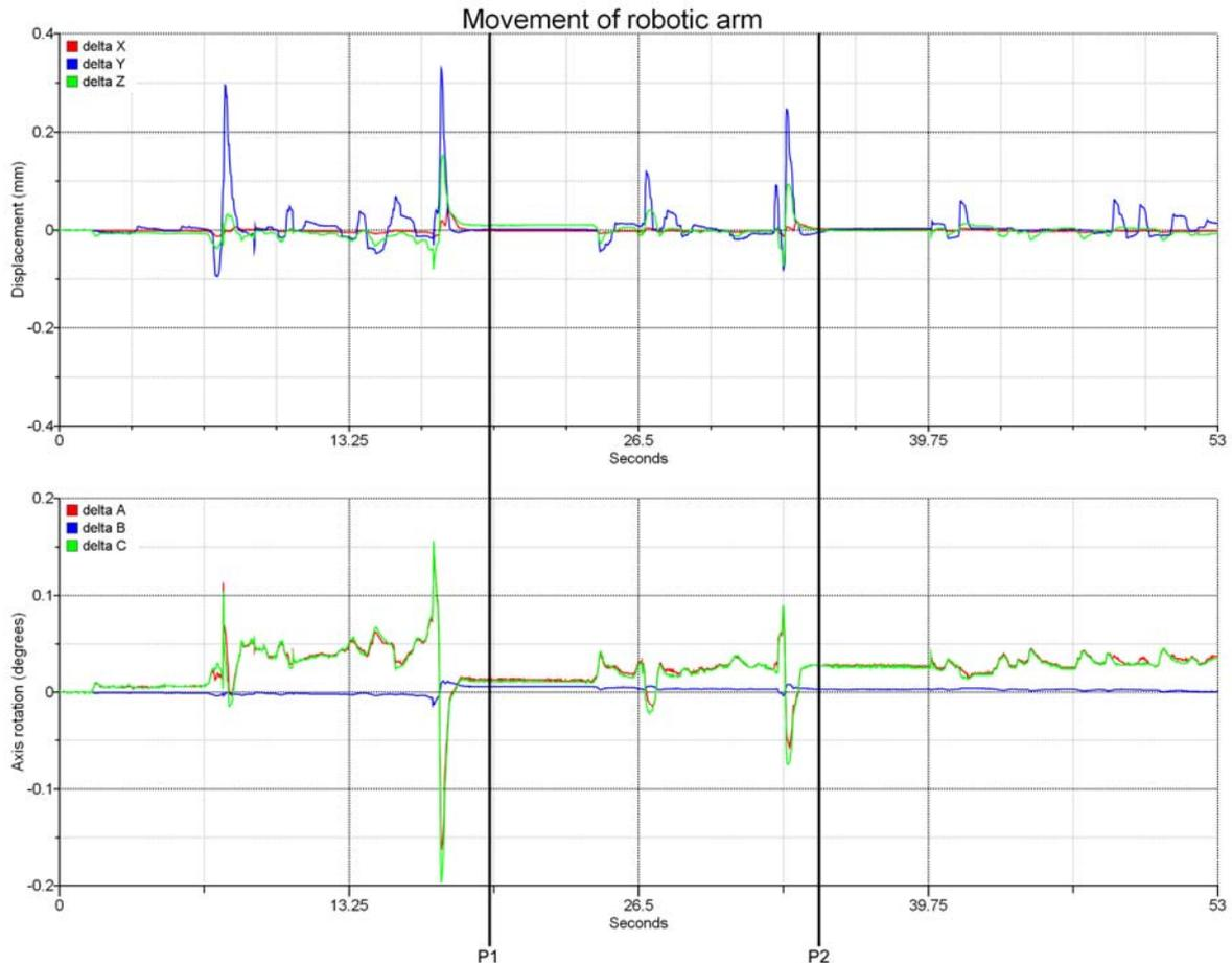
**Figure 84 - Robot arm position during drilling of the swine bone. Horizontal axis displays time in seconds. On the top graphic the vertical axis displays the robot arm displacement in millimetres, the bottom graphic the robot arm displacement in degrees.**
