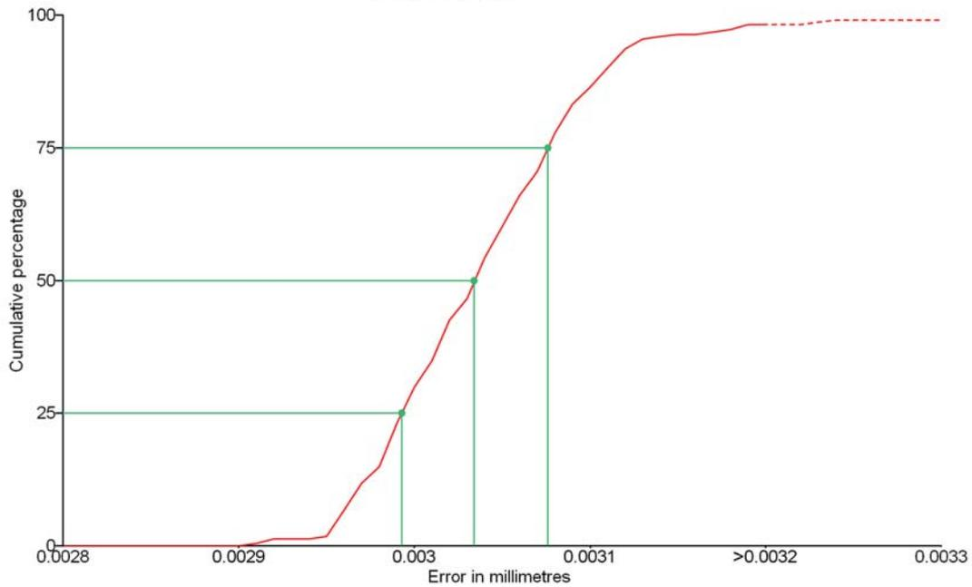
**Figure 77 - Cumulative XY position error within the tracking volume. Horizontal axis contains the error magnitude in millimetres. Vertical axis contains the cumulative percentage of the error.**
