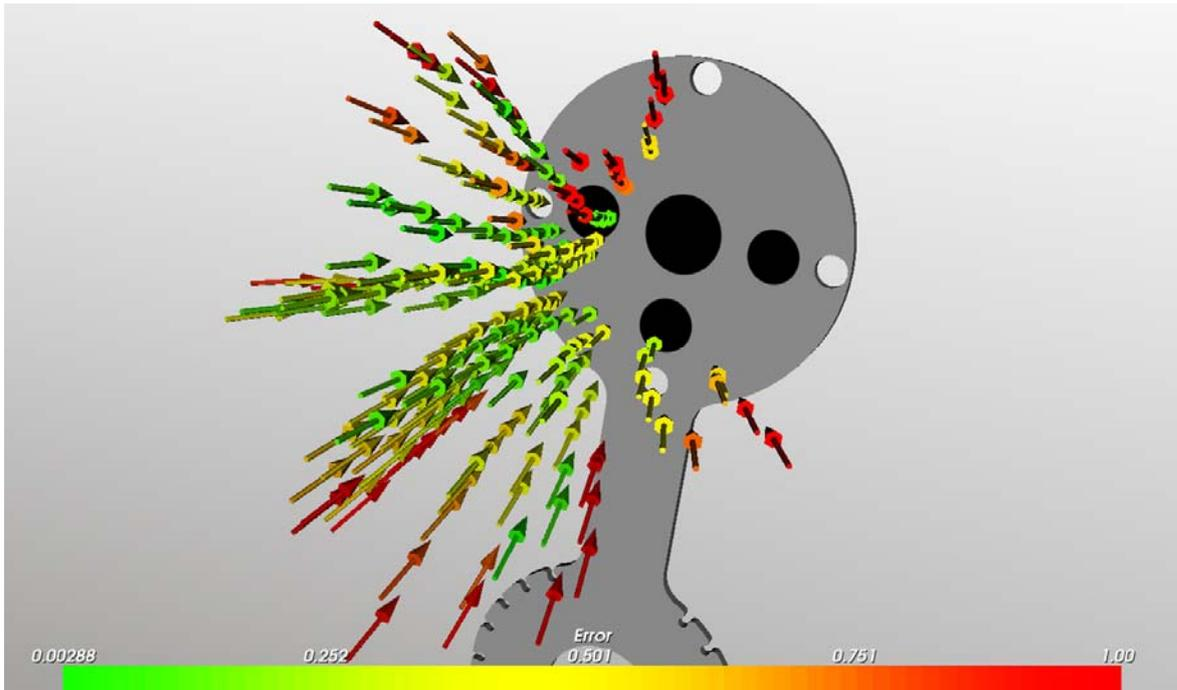
**Figure 76 - Spatial representation of the angle error growth with the camera distance and orientation.**
