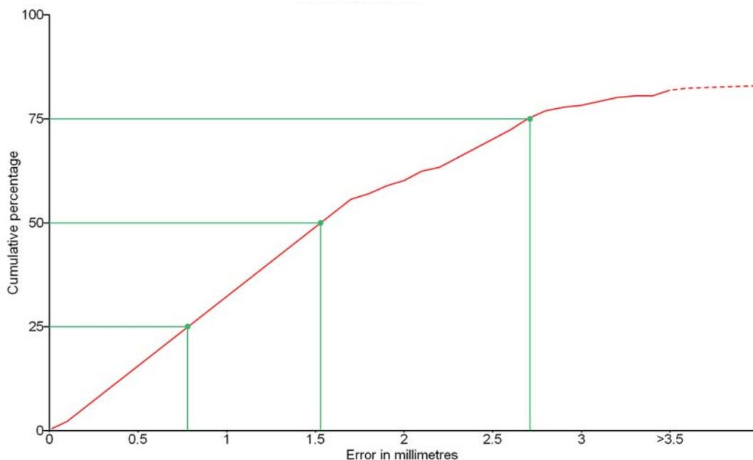
**Figure 73 - Cumulative depth error within the tracking volume. Horizontal axis contains the error magnitude in millimetres. Vertical axis contains the cumulative percentage of the error.**
