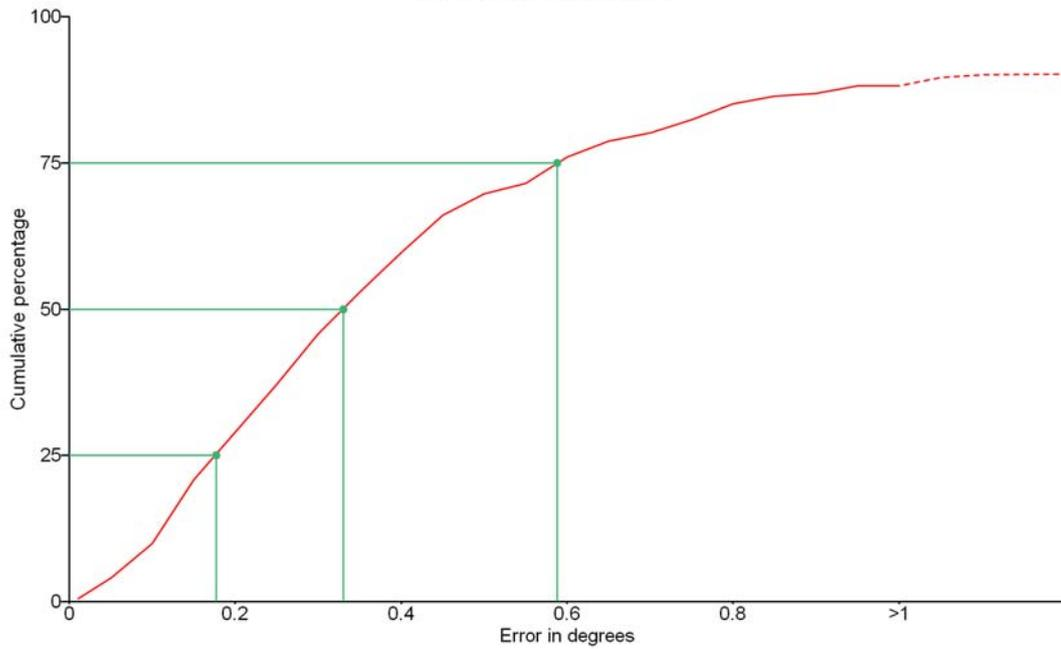
**Figure 75 - Cumulative coplanar angle error within the tracking volume. Horizontal axis contains the error magnitude in degrees. Vertical axis contains the cumulative percentage of the error.**
