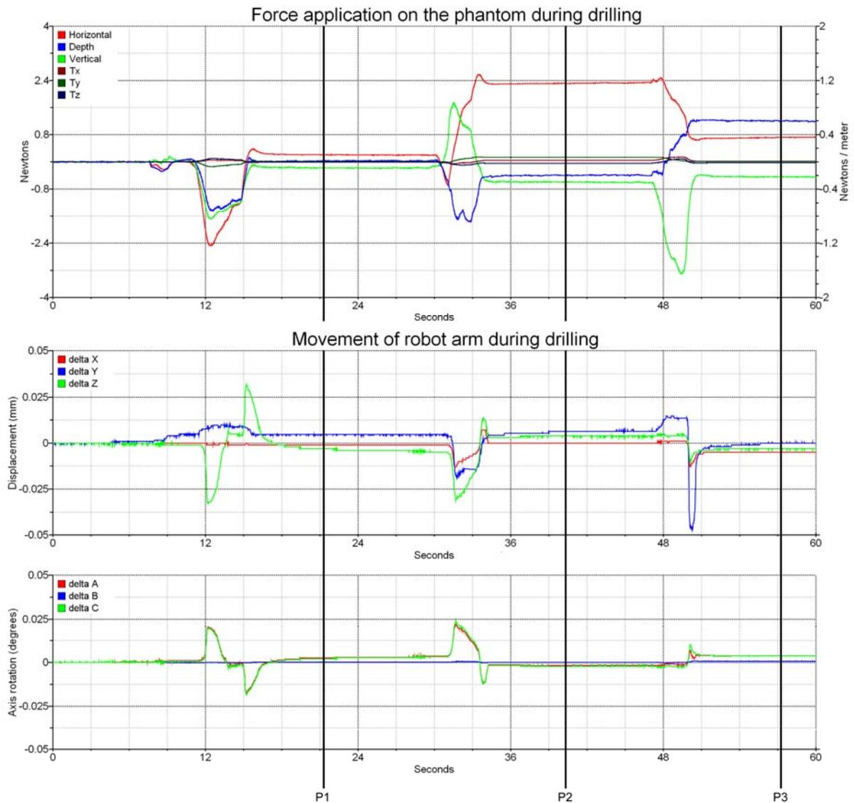
**Figure 83 - Robot position oscillation and applied forces during drilling of the phantom’s maxilla. Horizontal axis displays time in seconds. On the top most graphic the vertical axis displays measured forces in Newton as well as the torques in Newton / metre. The central graphic displays the robot arm displacement in millimetres, the bottom graphic the robot arm displacement in degrees.**
