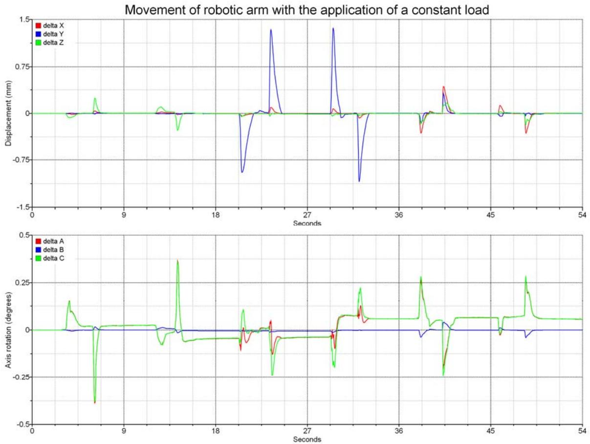
**Figure 81 - Top: Position oscillation with constant load applied. Down: Angle oscillation with constant load applied. Horizontal axis displays time in seconds. On the top graphic the vertical axis displays the robot arm displacement in millimetres, the bottom graphic the robot arm displacement in degrees.**
