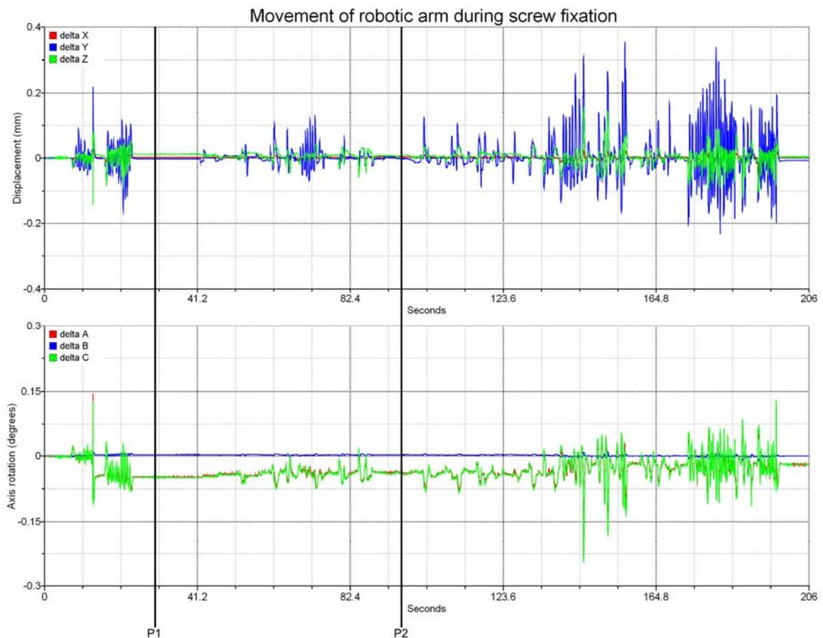
**Figure 85 - Robot arm position during screw fixation of the swine bone. Horizontal axis displays time in seconds. On the top graphic the vertical axis displays the robot arm displacement in millimetres, the bottom graphic the robot arm displacement in degrees.**
