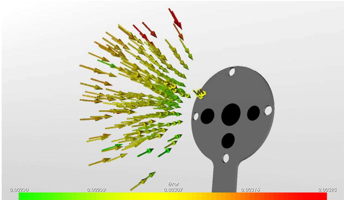
**Figure 78 - Spatial representation of the XY plane position error growth with the camera distance and orientation.**
